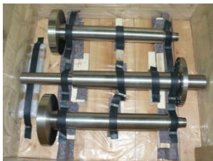
Shafts for drive unit and support rolls.
